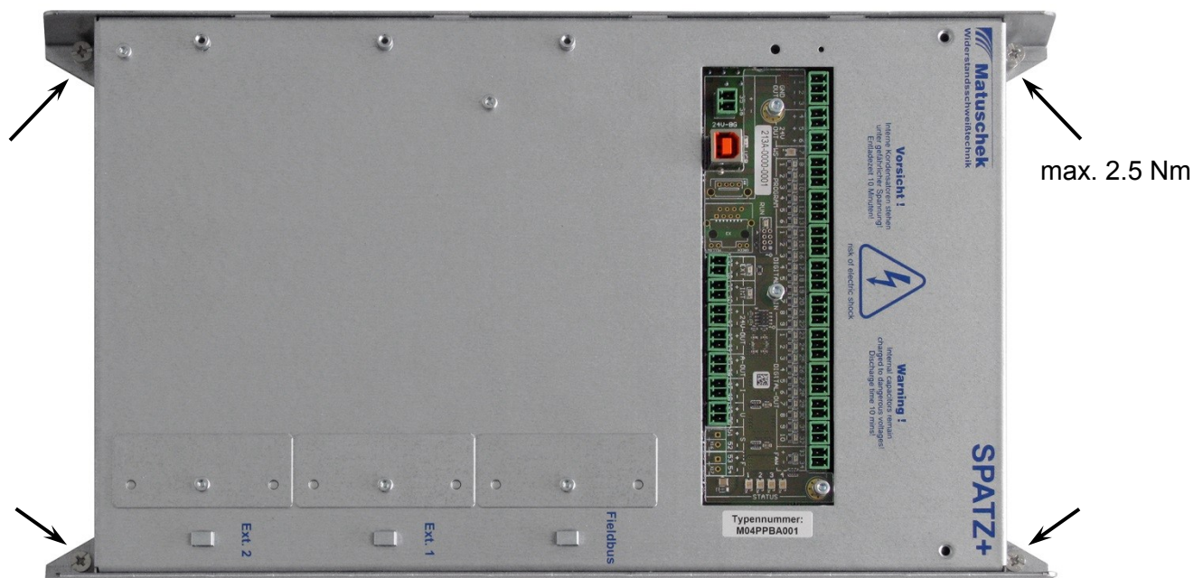
Figure 21: Position of fastening screws for exchanging the board set of the SPATZ+
